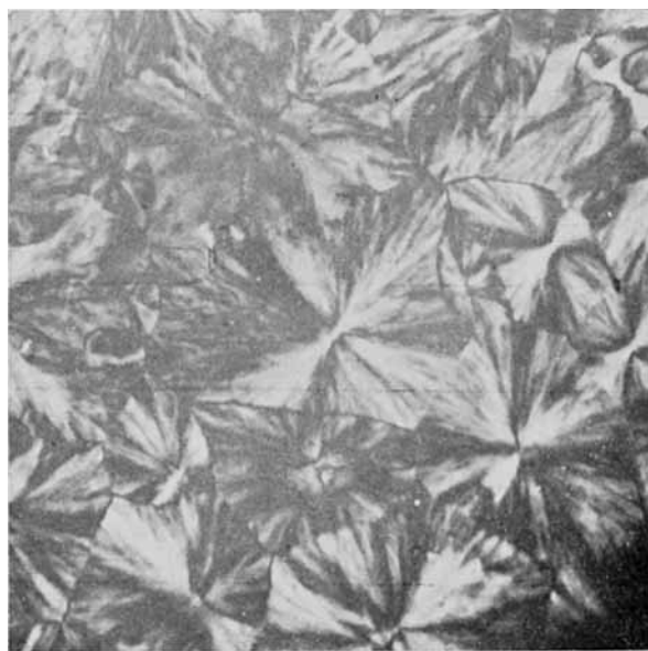
Fig. 5. Photomicrograph of high melting poly-4-MP prepared by sequential addition techniques; no annealing.
